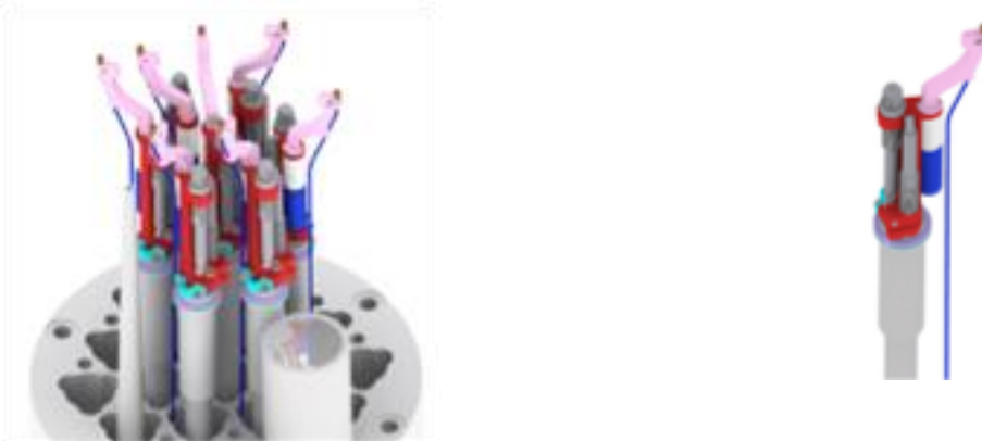
Fig 2: Fiber positioner design in MOONS focal plane.
